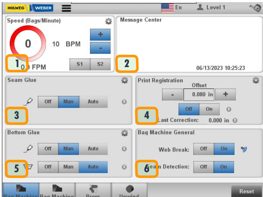
FIGURE 10. BAG MACHINE PRODUCTION TOUCH-SCREEN WINDOW FUNCTION DESCRIPTIONS
