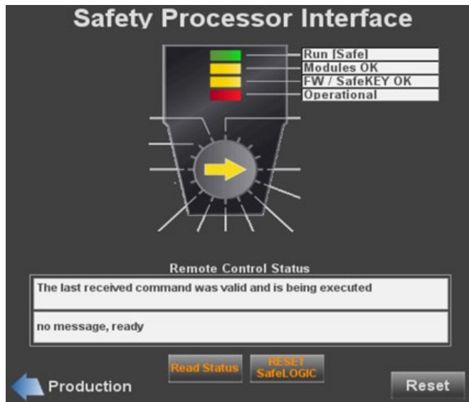
FIGURE 34 SAFETY PROCESSOR INTERFACE SCREEN
